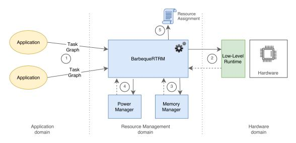
Figure 1: The MANGO partition-based resource management: (1) the applications provide their task graphs to BarbequeRTRM that (2) requests available partitions to the low-level runtime, then (3) (4) it asks to memory and power managers to skim the partition list and to assign a score to each partition. Finally, it selects the best partition and enforces (5) the resource assignment.
